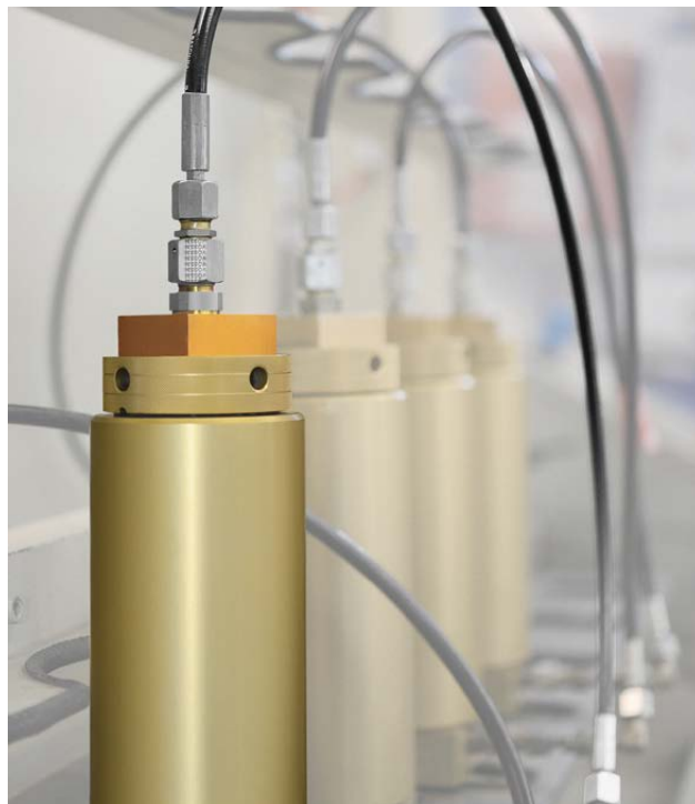
Pressure testing of filter housings
