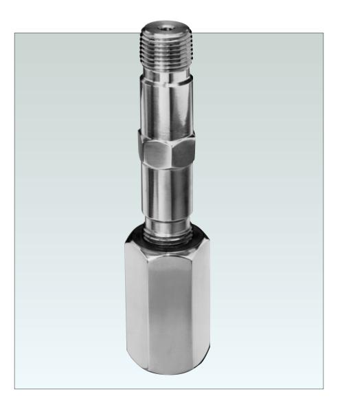
Use of the H7H Valve in connection with the Gauge Siphon further reduces the gauge temperature by lengthening the condensate leg. The condensate will then 'hang-up' between the valve orifice and the top of the 1/4-inch tube. That is, condensate will also occupy the lower part of the Siphon.
