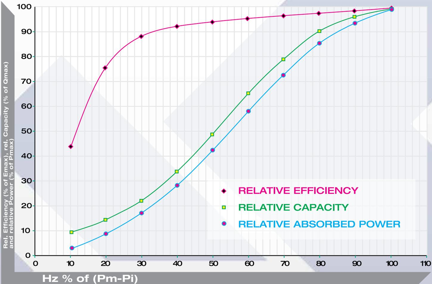
PREFABRICATED COMPACT SCREW PUMPS
