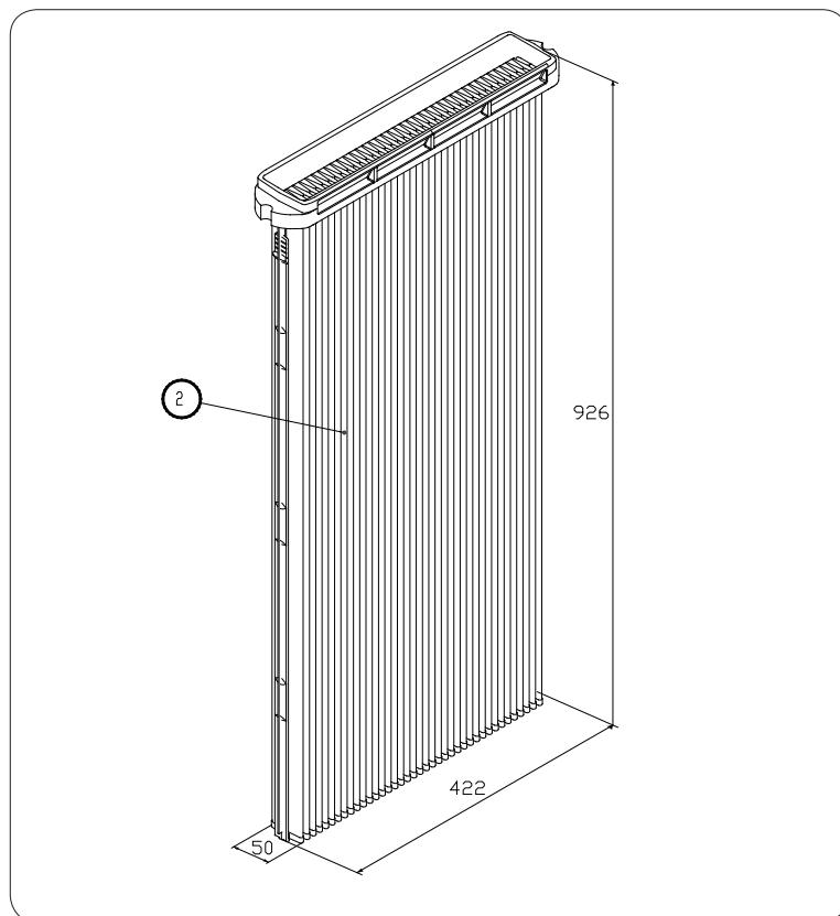
The SILOTOP® R03 Venting Filter is provided with seven POLY- PLEAT® filter elements. These elements are parallelepiped-shaped and the dimensions are as shown in the diagram above; the filtering medium is a non-woven pleated spunbonded fleece with B.I.A. class M certification.. The total filtering surface is 24.5m<sup>2</sup>.
