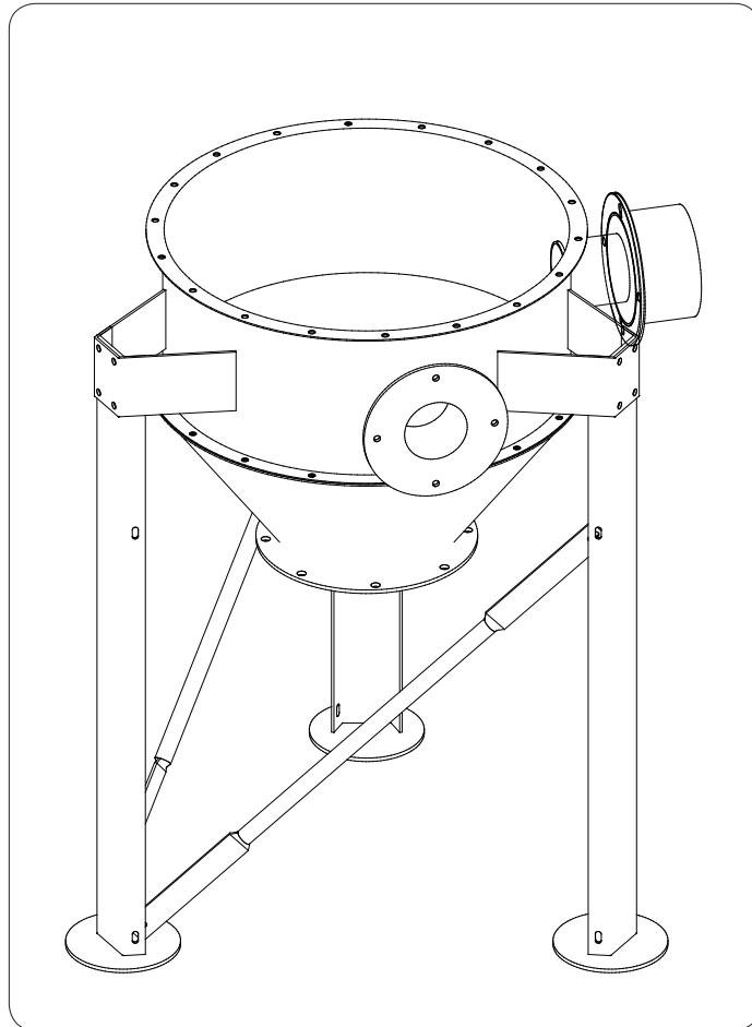
If it is found to be necessary to check the SILOTOP®R03 filter emissions (basic supply) a special kit is available for conveying all the air from the filter outlet into a single pipe.
