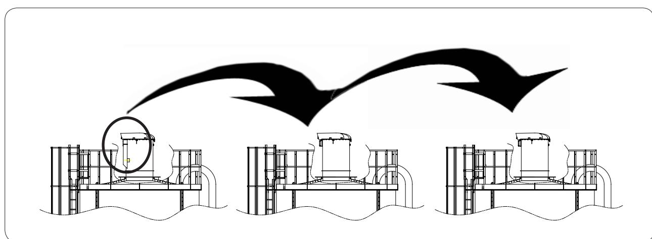
In case of plants with many filters, WAM® suggests using a single tube to be shifted from one filter to another.
